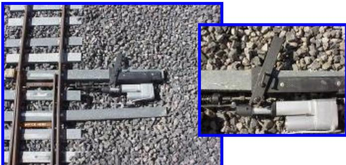
Art Crisp has designed a very clever feature for the new switch machines now in use at Train Mountain. It is an **override**. This **override** allows you to override the current setting of the switch machine. Move the lever shown to the desired position and then turn the bolt to set the switch in that position. Once clear, simply undo the bolt to return the machine to the correct position. Very cool! Thanks Art!
