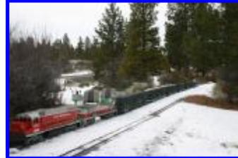
The first couple of trips met with some challenges. Frequent stops were required to restack the ties on to the cars. Turns out the oily rail and the plastic ties made for some slippery panels.
