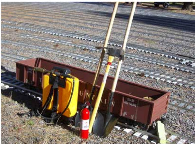
These gondolas can and should be added to trains at the lower levels of fire danger. As experience has illustrated to us fires can start at the lowest levels of Fire Danger. All Work Trains should add one of these cars to their consist. We are also adding the required firefighting equipment to all Train Mountain Vehicle's. We will be enhancing the fire equipment on the Gators with an additional Indian Manual Back Pump holding 5 gallons of water.
