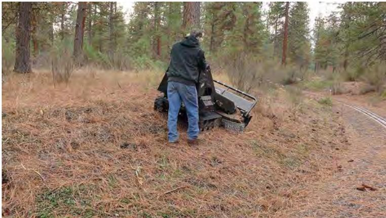
In this image, Richard is demonstrating how well the Brush Blazer does running along a side-hill. There is a limit, as at some point you tend to slide sideways down the hill. The alternative is to then run the Brush Blazer up and down the hill, but this is a lot more work and not nearly as efficient.
