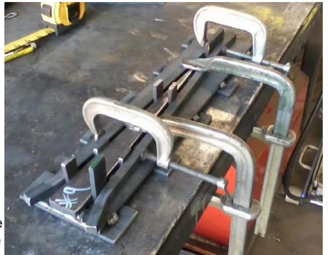
The rest of the parts are cut from 1/4" x 2" strap steel, 1/2" x 1/2" square steel bar stock and 1/4" x 1- 1/2" strap steel. This stock is cut to size on a band saw, deburred and made ready for welding. Laying out of the parts for welding is accomplished by using some 1/4" spacers and a careful placement of the frog heel and securely clamping into place (see accompanying photo). Once welding is completed the frog is ready for installation.
