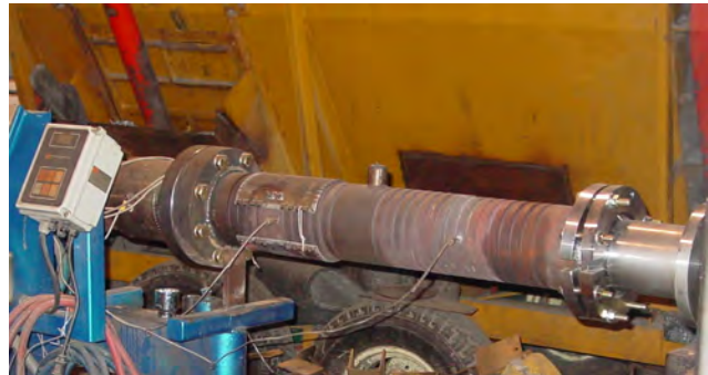
Above -- Feeder Tube electrically heated to keep the plastic hot & flowing.
