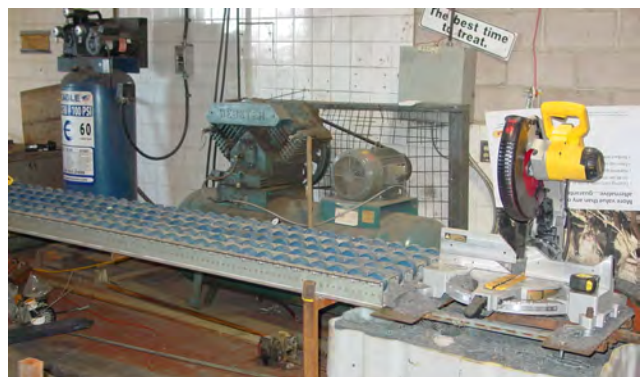
Right -- 8' Tie are cut to 16" lengths with standard chop saw.
