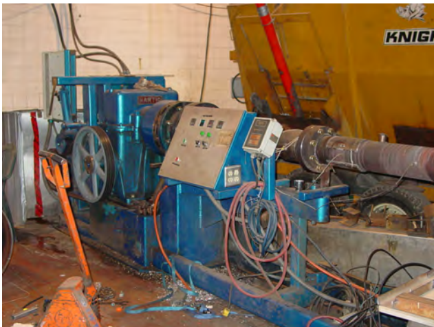
Above -- Plastic Chips are heated, compressed, and pumped hot into Feeder Tube.
