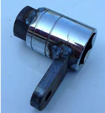
In the Switch Stand box install the socket with its wing in the clevis fork with a clevis pin and cotter pin.
