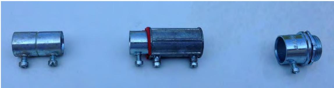
We use metal conduit for the tube. The 3/4" metal conduit connector (right in the photo) connects 5 feet of 3/4" metal conduit to the Grey Metal Boxes. A 3/4" to 1/2" conduit connector (center in photo) connects a 10' piece of 1/2" conduit. Then 2 more 10' pieces of 1/2" conduit are connected with 1/2" conduit connectors (left in the photo). Then step back to a final 5 feet of 3/4" conduit. So the order of assembly is 5'(3/4), 10'(1/2), 10'(1/2), 10'(1/2), 5'(3/4). I take care to make all the
