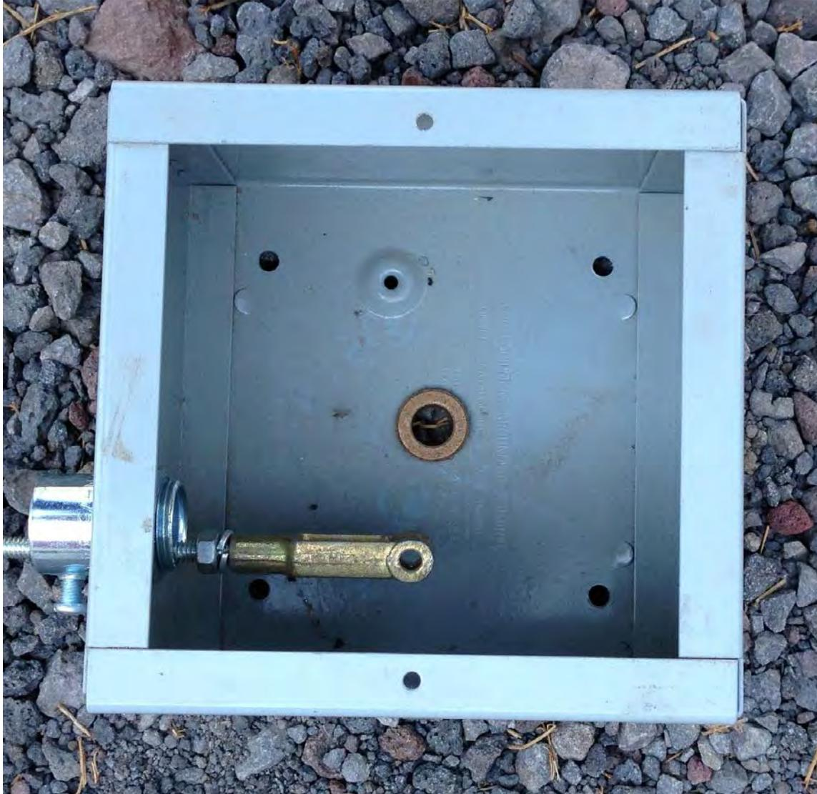
Then adjust the rod/clevis forks or rod length so the clevis pin lines up with the holes in the center of the top of both the boxes.
