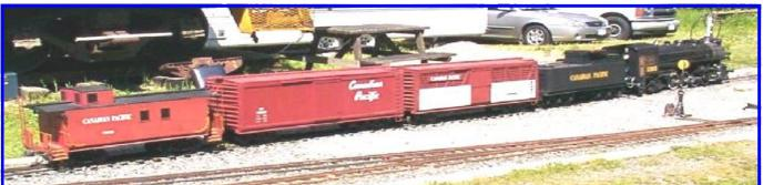
C.P.R. 5303 Engine & Tender, Cattle car (gas car) Box car (bench type riding car) Caboose (equipment car). The engine burns all three fuels, coal, diesel oil and propane, change over takes about 20 minutes. First run June 1998.
